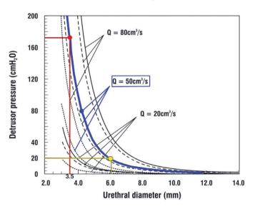
**Figure 3.** Pressure flow graph - detrusor pressure as a function of urethral diameter for urethral length of 4 cm at flow rates of 20, 50, 80 ml/sec (8). Total resistance to flow (unbroken line) — Frictional component ...... Dynamic component - - - - . For a flow rate of 50 ml/sec (blue line), increasing the diameter of the urethra from 3.5 mm to 6 cm, reduces the head of pressure required to empty from approximately 170 cm H<sub>2</sub>O to 20 cm H<sub>2</sub>O. *Q: Flow (cm<sup>3</sup>/s)*
